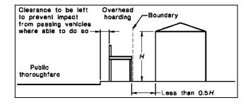
The Principal Contractor or Owner-builder must ensure that overhead protective structures are installed and maintained in accordance with the NSW "Code of Practice - Overhead"
